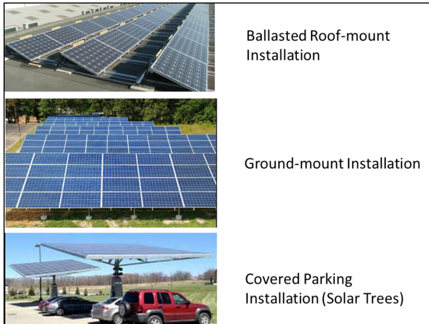
Figure II-I – PV Installation Options.
